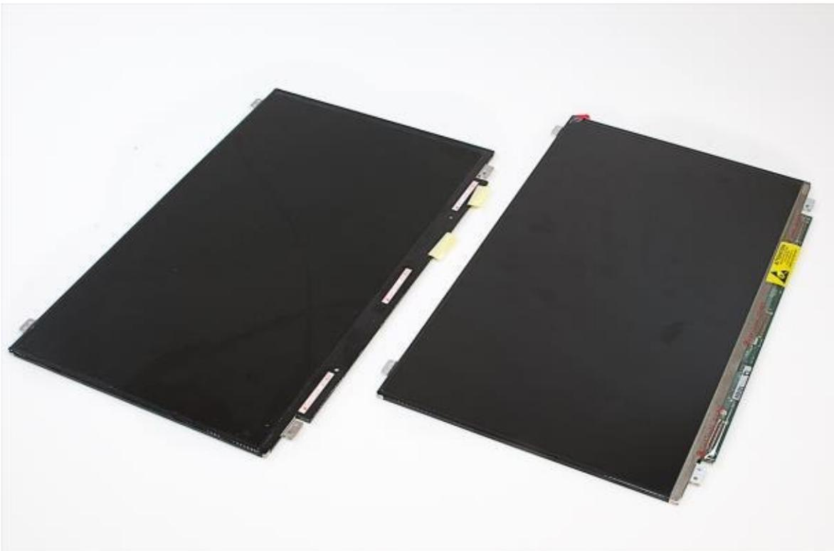
the dimensions, mounting brackets, and connector all match, you ready to install the screen. Connect the new panel to the cable, position the panel in the lid, and secure it
