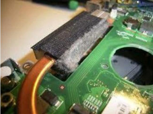
between the fins of the heat-sink, remove all dust and debris from the heatsink. You will then need to unscrew or un-brace the fan from the heat-sink to properly clean the fan. These will be micro sized screws typically 4 of them and some might be hidden under plastic stickers.
