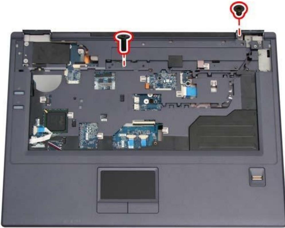
3. Turn the computer over again and disconnect the power USB board FFC, touchpad, and finger printer cables as shown.
