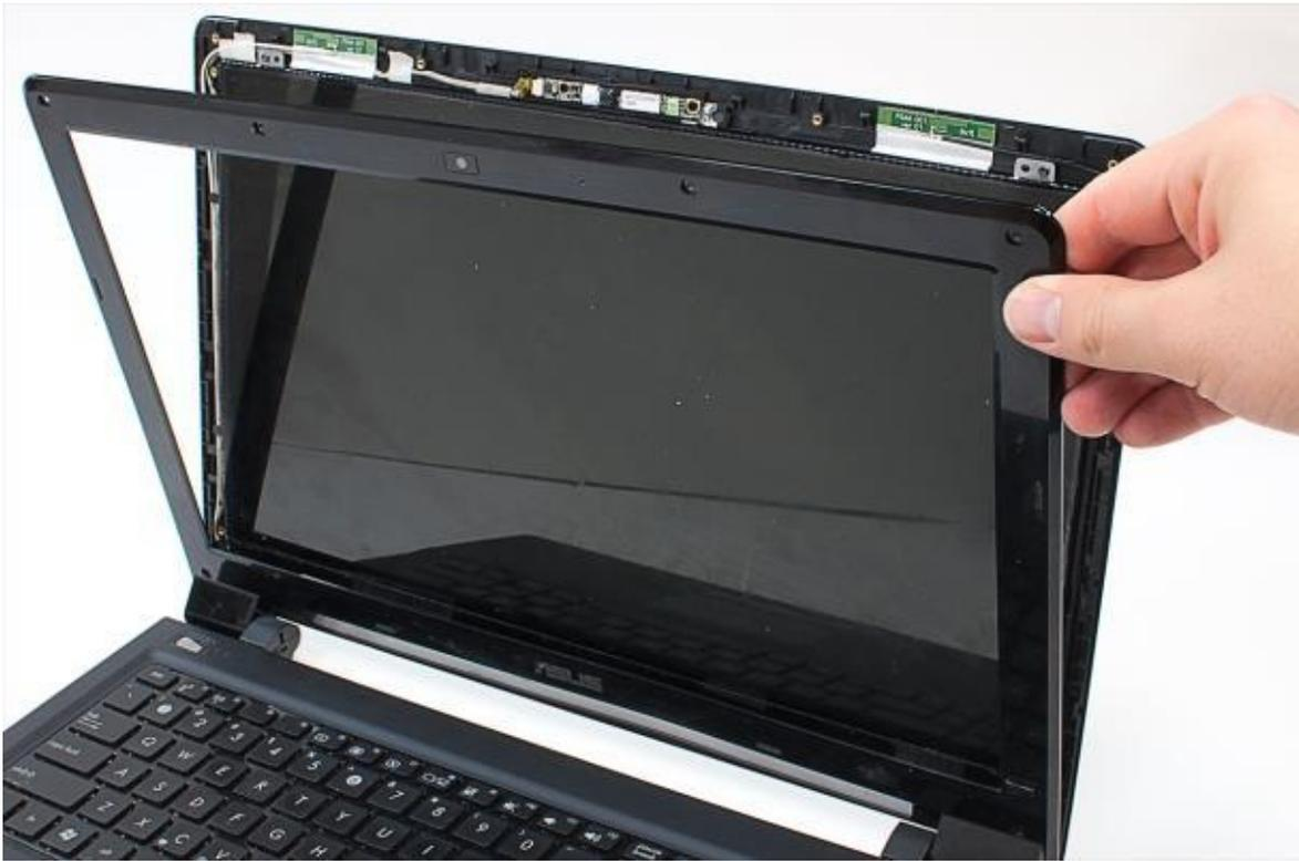
**2. Remove the broken LCD panel :** With the LCD's mounting brackets exposed, you can remove the screws that secure it to the lid. Then rest the display front-side-down on the case and disconnect its cable.
