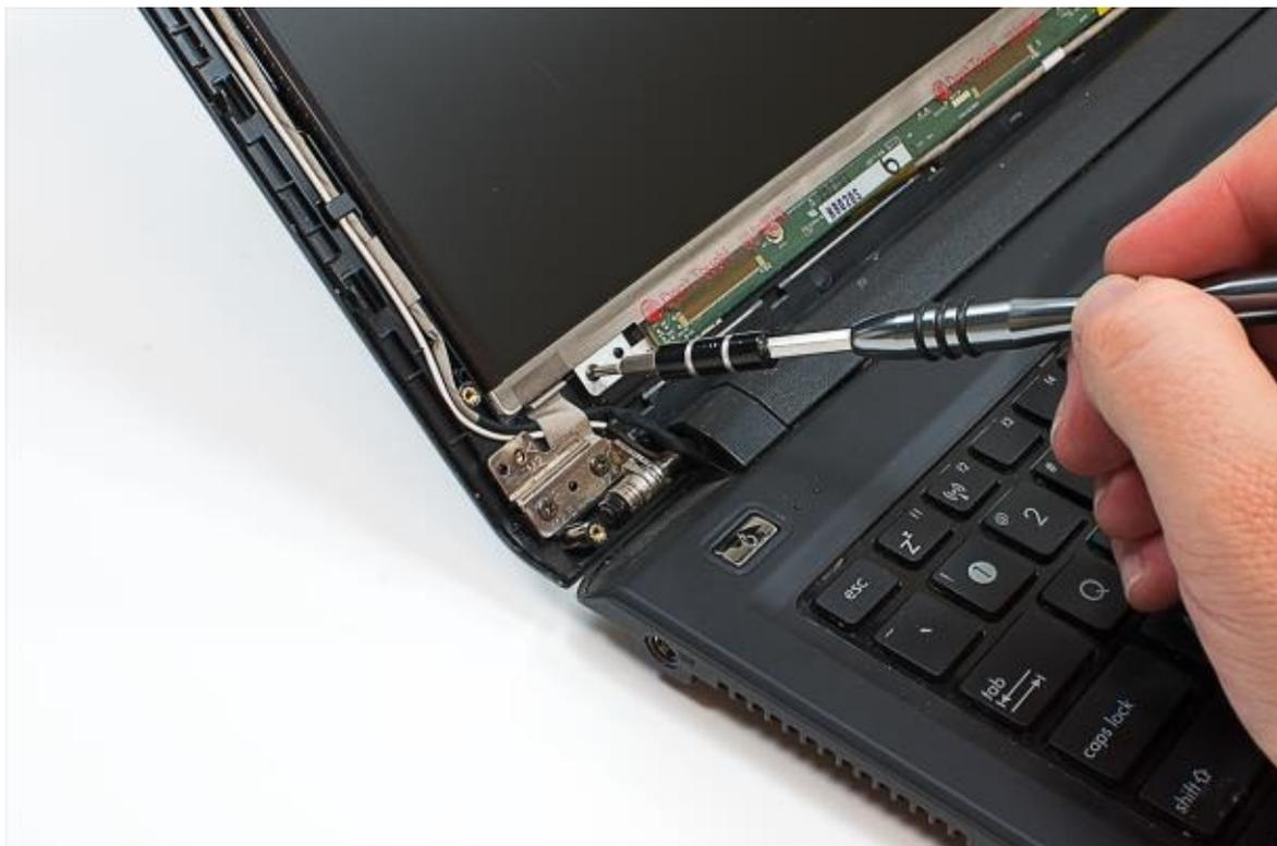
**4. Test the new LCD panel and reinstall the bezel :** Before reattaching the bezel, it's a good idea to test the new panel. Reconnect the battery and power cable and turn the machine on. If the display works, you can reattach the bezel and any external screws and rubber cushions. The repair is now complete.
