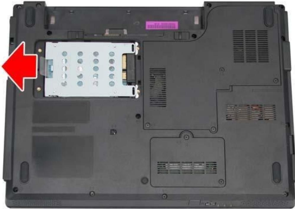
6. Remove the four silver M3x3 screws to take off the HDD case.
