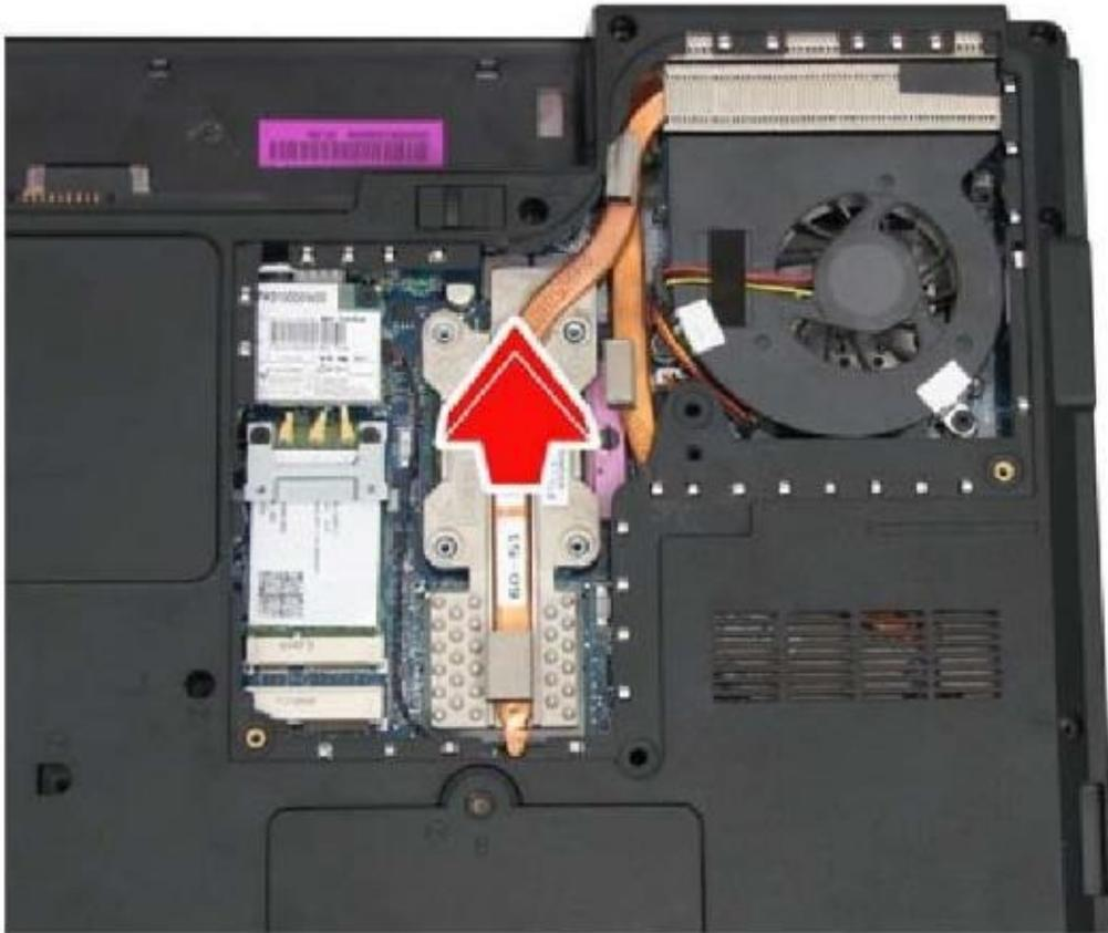
**CAUTION:** When you remove the thermal module, use the CPU grease tool to remove the grease on the CPU and thermal module. Reapply fresh grease before reinstalling the thermal module.
