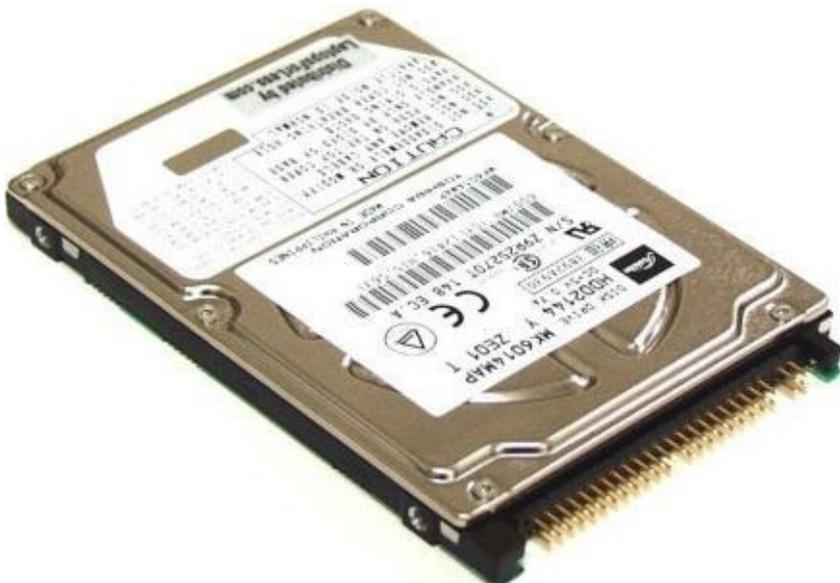
if the hard drive had any issues with it that were stopping the laptop from powering on, removing the drive should bypass the issue and allow the laptop to turn on. Liquid damage to the hard drive is a common reason this can happen... Liquid damage to the internal components can cause
