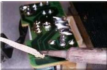
copper visible in the portion that is removed: braid is very expensive.
