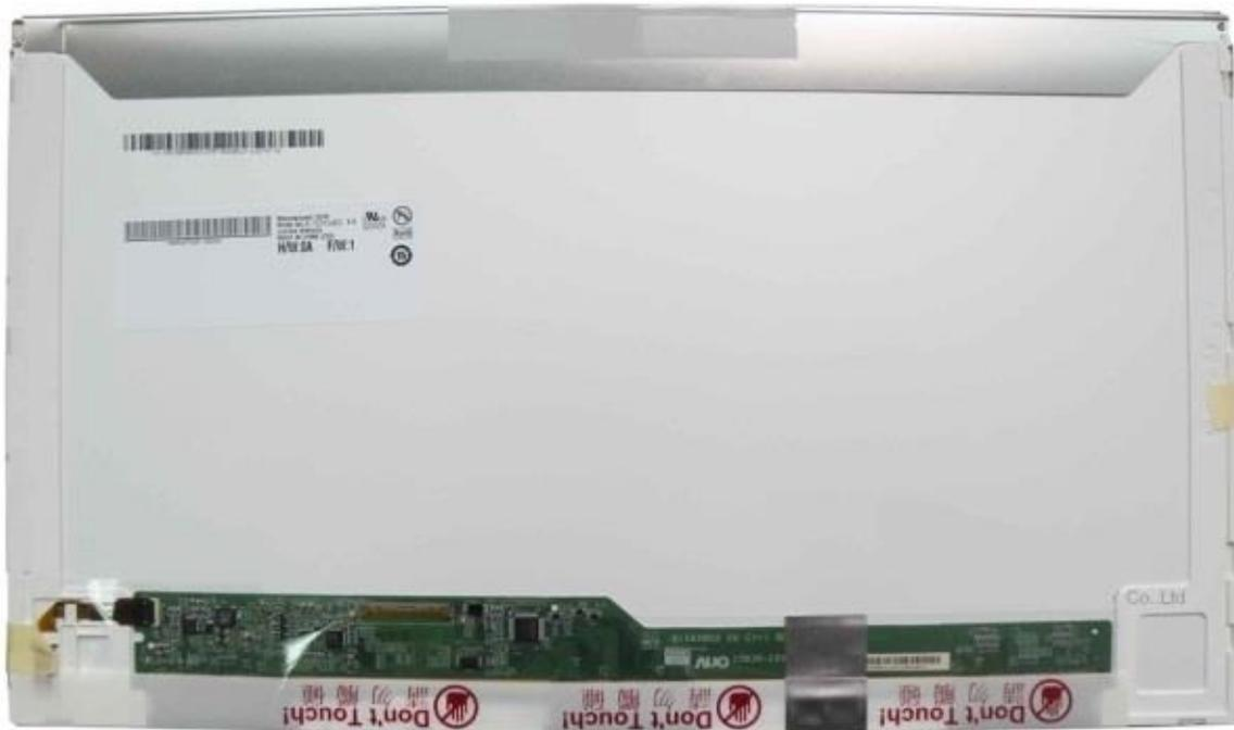
This is located in the display panel and will be found on the bottom end of the screen stretching from the right end to the left end...The CCFL
