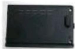
separately. For instance, the hard drive will have its own cover, usually secured by 2 or 4 screws, Wi-Fi card access bay will sometimes have its own cover too. The RAM DIMM slots are always accessible from case covers and will usually have their own cover. Some laptops will combine the covers into 1 large cover or 2 separate larger covers.
