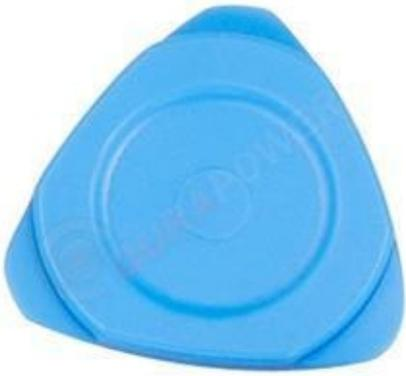
able, you will ALWAYS use plastic over metal to disassemble or work on the laptop or any electronic component. There are various kinds that are used and needed. A guitar pick is the most used tool, not a flimsy pick rather a slightly thicker guitar pick that can withhold
