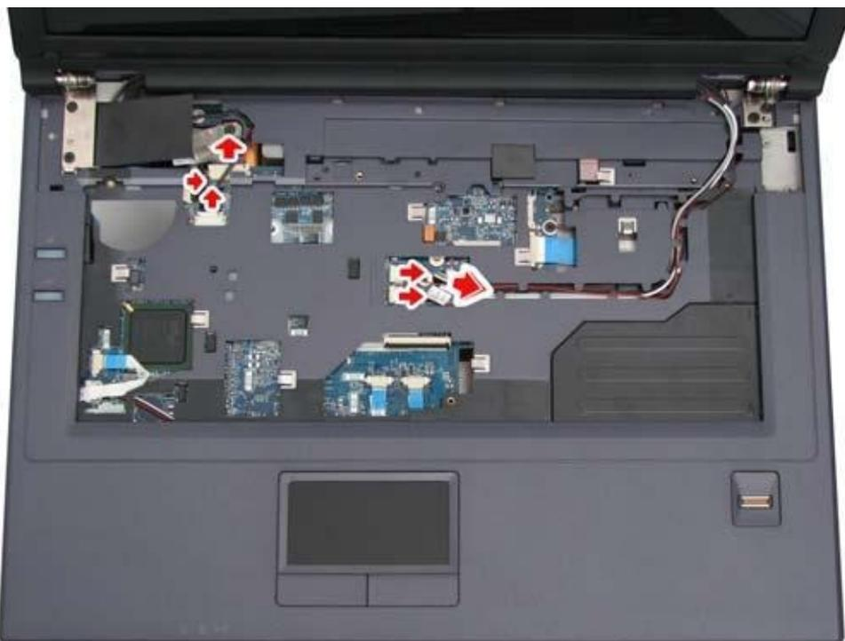
2. Remove the four M2.5x4 screws securing the LCD module to the logic upper.
