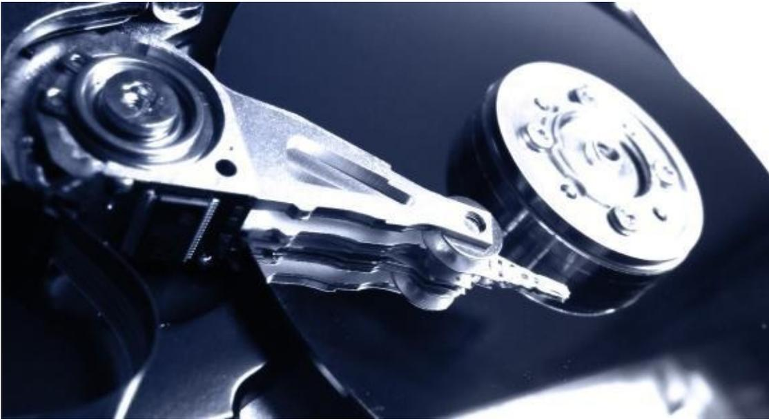
The damage can be either internal or external. A clicking sound, for example, is suggestive of a malfunctioning head, i.e. internal damage. A completely dead drive, on the other hand, could be due to a faulty printed circuit board (PCB), which would be external damage.
