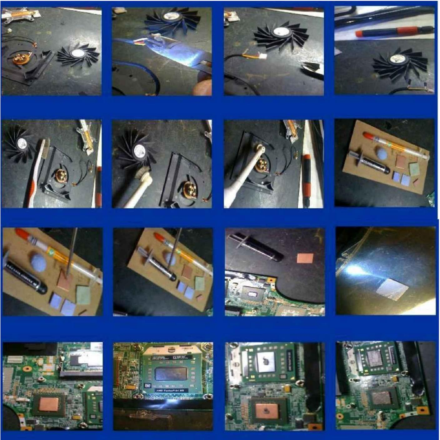
The CPU will always use thermal paste because it does not get as hot as the GPU does. The GPU will almost always use a thermal pad and not paste. Thermal pads will allow for the natural thermal expansion of the chipset and will allow for the greatest heat dissipation. Do not replace the thermal pad with a copper shim on a NVidia chipset... You must reuse the thermal pad on the video chip.
