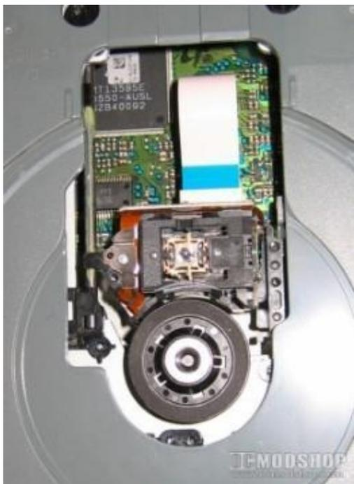
much dust or debris in it, so be sure to clean out the inside with either compressed air, a soft cloth, or a cotton swab. Reassemble the disc drive, put it back in the computer case, and cross your fingers. Hopefully, it will work when you turn on the computer.
