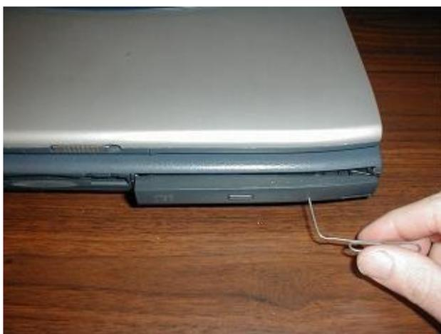
out when the paperclip pushed in the release, which you can tell by feel. So I had to pull on it with my fingernail behind the plastic facade while depressing the release. It opened pretty stiffly for the first fraction of an inch, and then pulled right out the rest of the way. That pretty much covers what you'll encounter with manually opening an optical drive, either it will pop open as soon as the paperclip works the latch, or you'll have to help it along.
