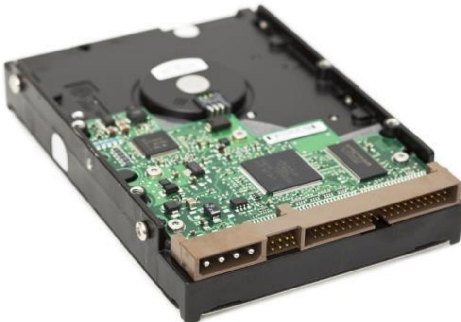
Even if you can see that your PCB is damaged, there might still be internal damage. Moreover, as mentioned above, replacing the circuit board yourself can damage your drive further, which reduces your chances of recovering your data.
