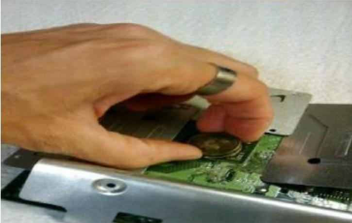
Once you have reached the correct temperature or time length , let the coin stack sit on top of the chip until cooled. Then remove the coin stack and this sheets/foil.
