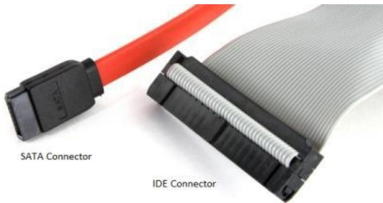
install the drive internally on your desktop computer. Alternatively, you can get an IDE / SATA to USB adapter or a new USB enclosure, so you can hook the drive up externally via USB.
