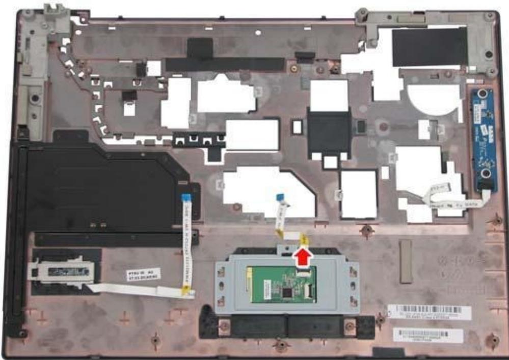
5. Remove the M2.5x4 screw securing the touch pad bracket to the logic upper. Lift off the bracket and remove the touch pad.
