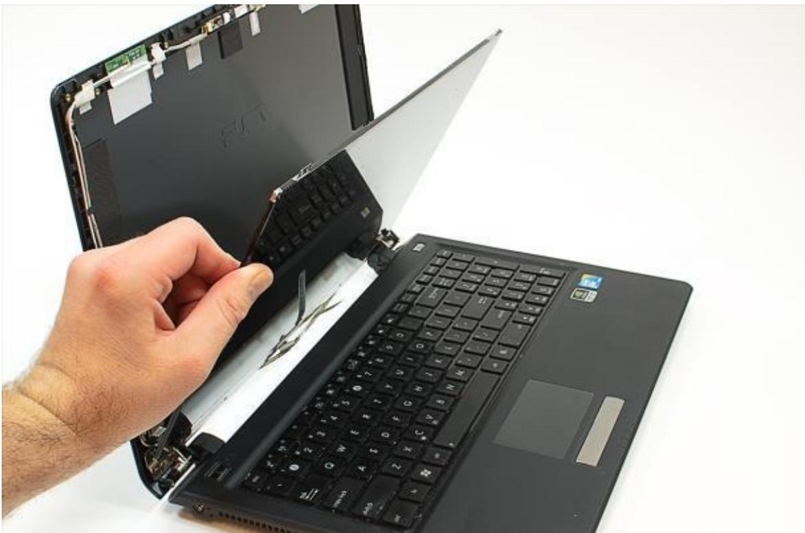
If your laptop was made before 2010 and has a LCD with fluorescent backlights, it will likely have two cables. But as this is an LED-backlit LCD, it only has one.
