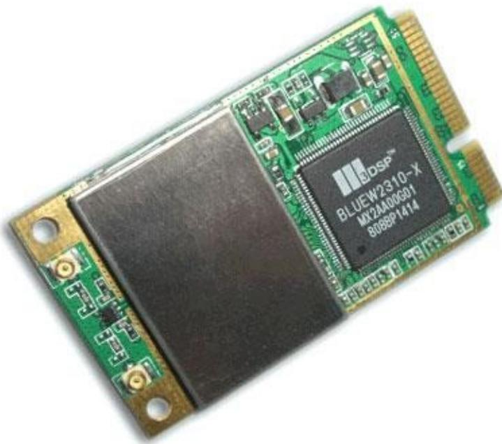
use for that specific laptop. It is ok to mismatch the color guide for the Wi-Fi antenna wires. Typically the wires are white and black, and will have colored arrows on the Wi-Fi card showing you what wire to connect to what site input plug. It is ok to plug the black onto the white port and visa versa as it will still
