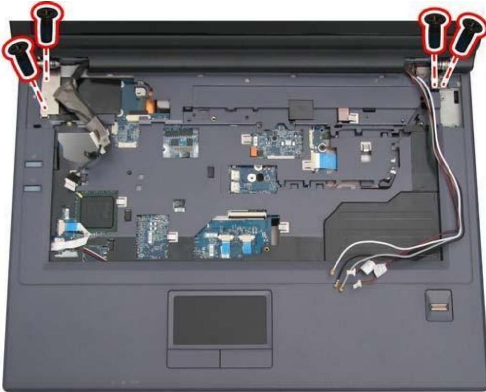
3. Remove the LCD module.
