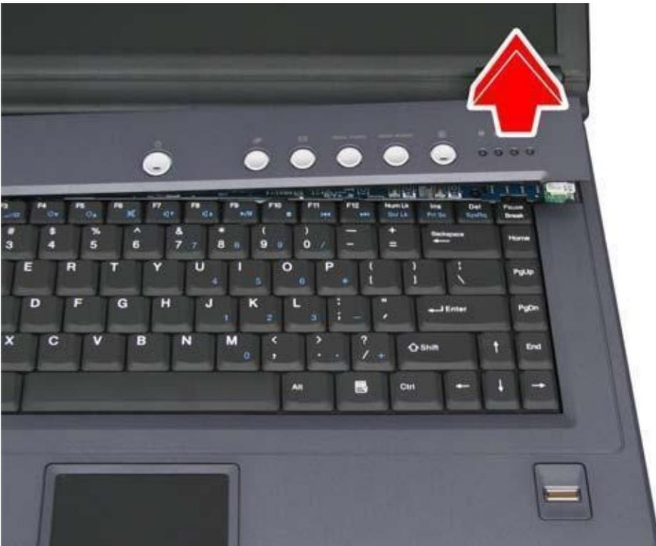
2. Remove the two M2.5x4 screws securing the keyboard. 3. Turn over the keyboard, revealing the keyboard cable underneath.
