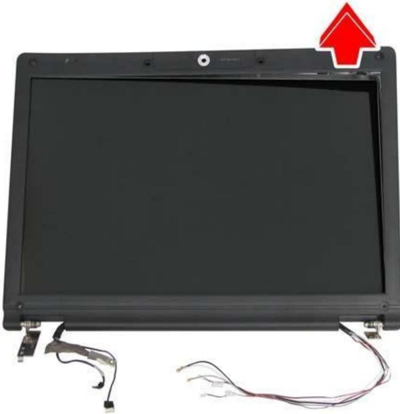
4. Remove the five screws mounting the display, inverter board, and LVDS/CMOS cable to the LCD cover.
