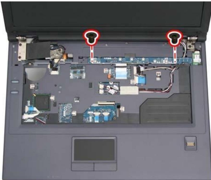
2. Remove the switch board.
