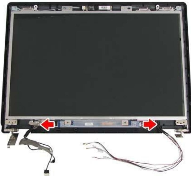
6. Gently lift out the display. Remove the eight M2x3 screws securing the hinges to the
