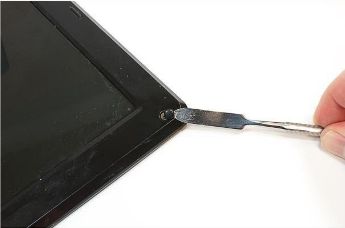
On this laptop, several rubber cushions hide screws, which hold the bezel in place. I'll need to remove these cushions and the screws that are underneath.
